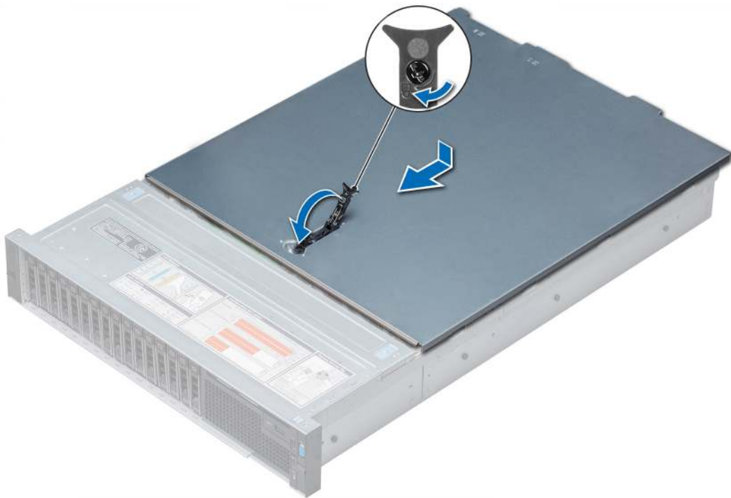
Figure 27. Installing system cover
