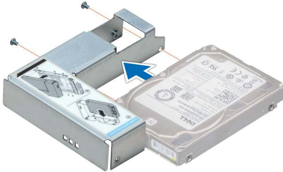
Figure 51. Installing a 2.5 inch drive into the 3.5 inch drive adapter
