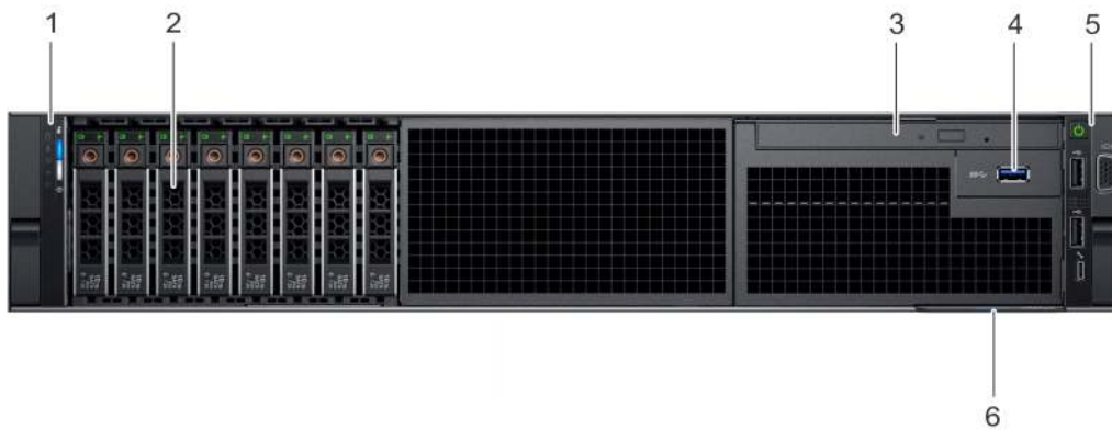
Figure 3. Front view of 8 x 2.5-inch drive system
