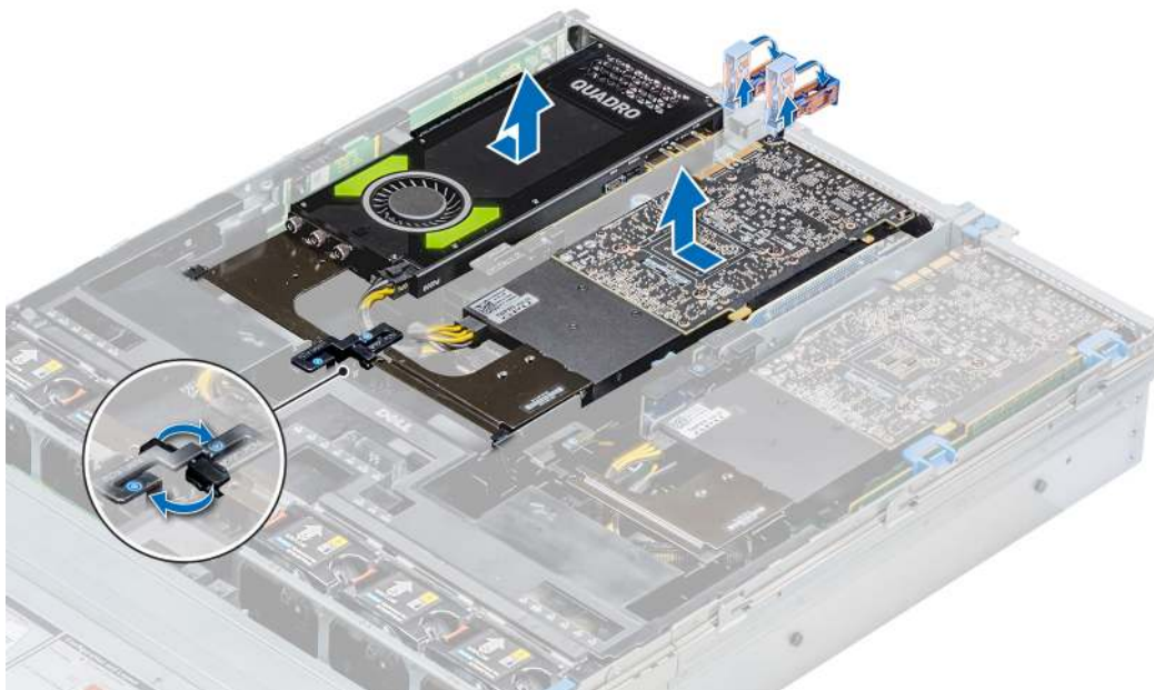
Figure 89. Removing GPU 2 and 3
