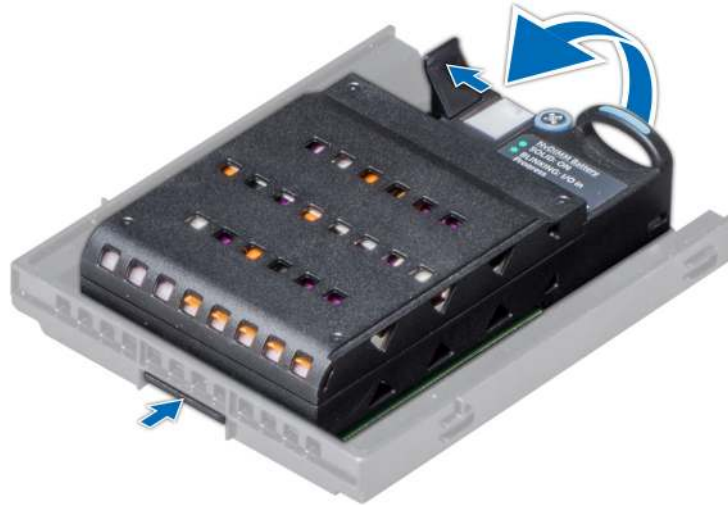
Figure 44. Removing NVDIMM-N battery from the bracket
