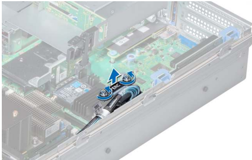
Figure 105. Removing integrated storage controller cable
