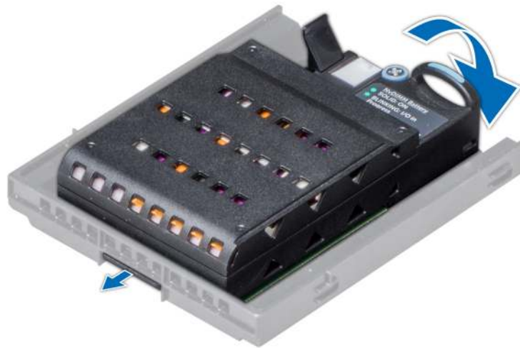
Figure 45. Installing NVDIMM-N battery into the bracket
