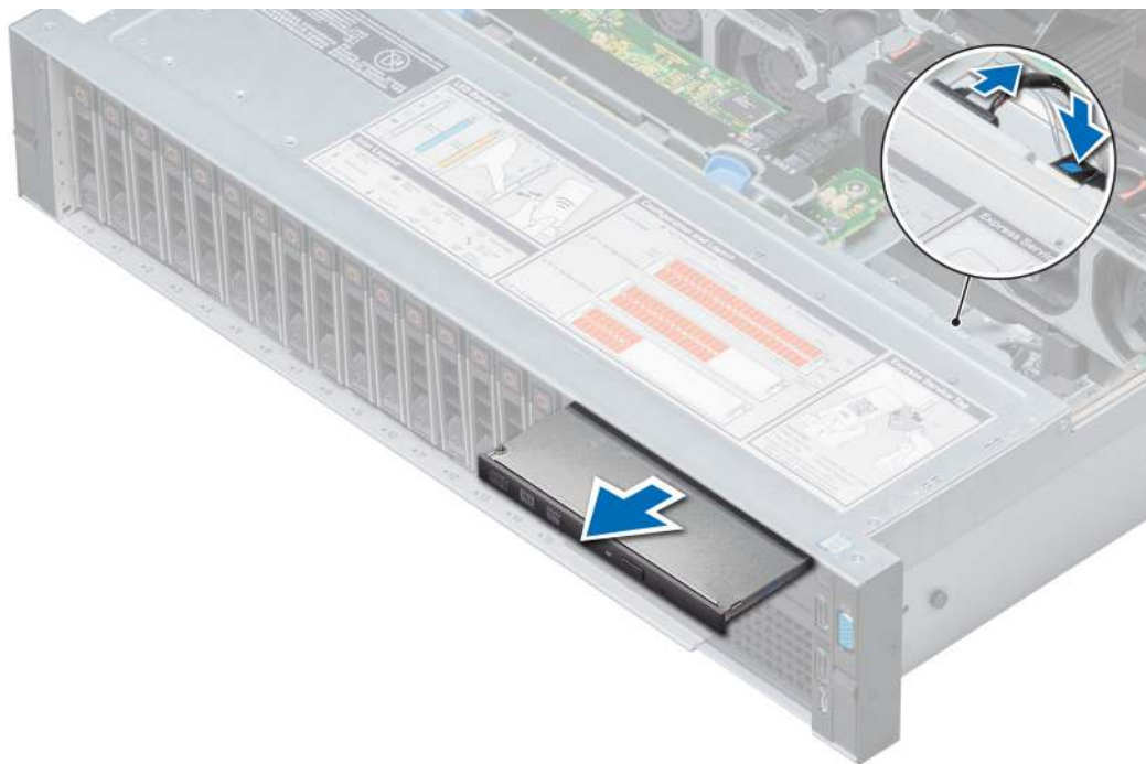
Figure 125. Removing the optional optical drive
