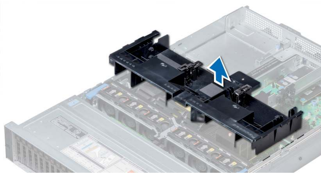
Figure 32. Removing air shroud
