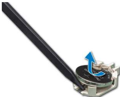
Figure 121. Removing the system battery
