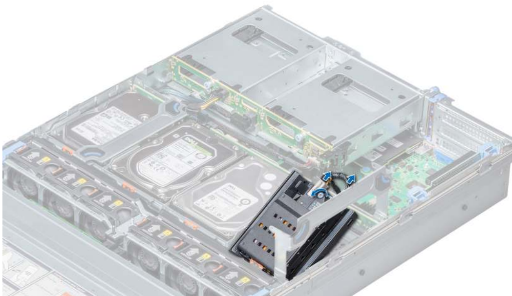
Figure 42. Removing NVDIMM-N battery from mid drive tray
