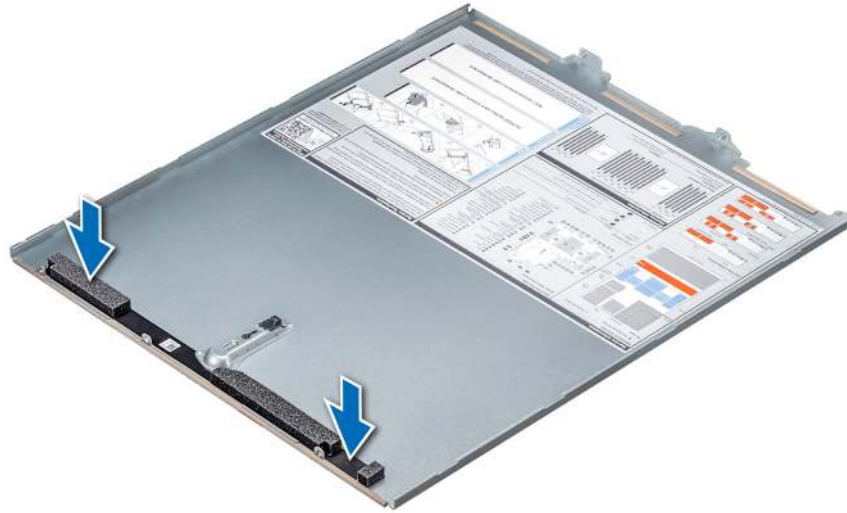
Figure 98. Installing mylar foam on the system cover
