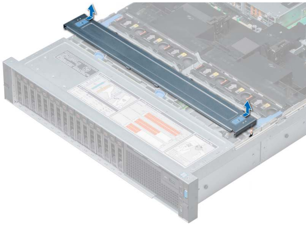
Figure 28. Removing backplane cover
