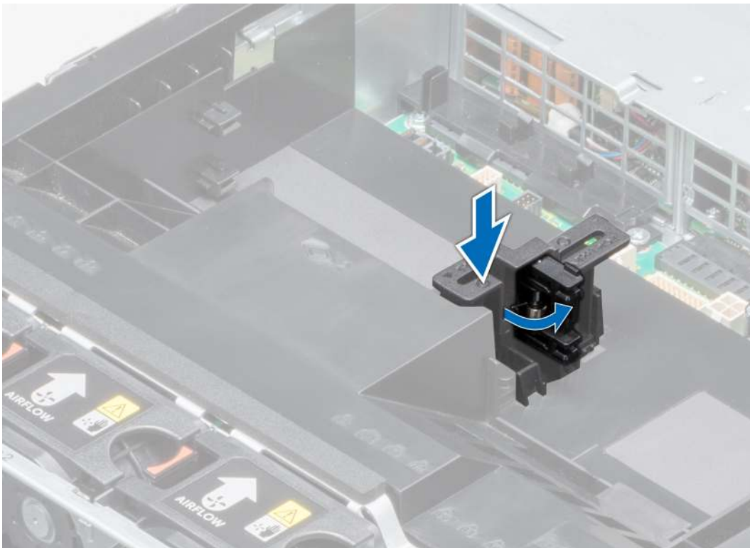
Figure 65. Opening the PCIe card holder latch
