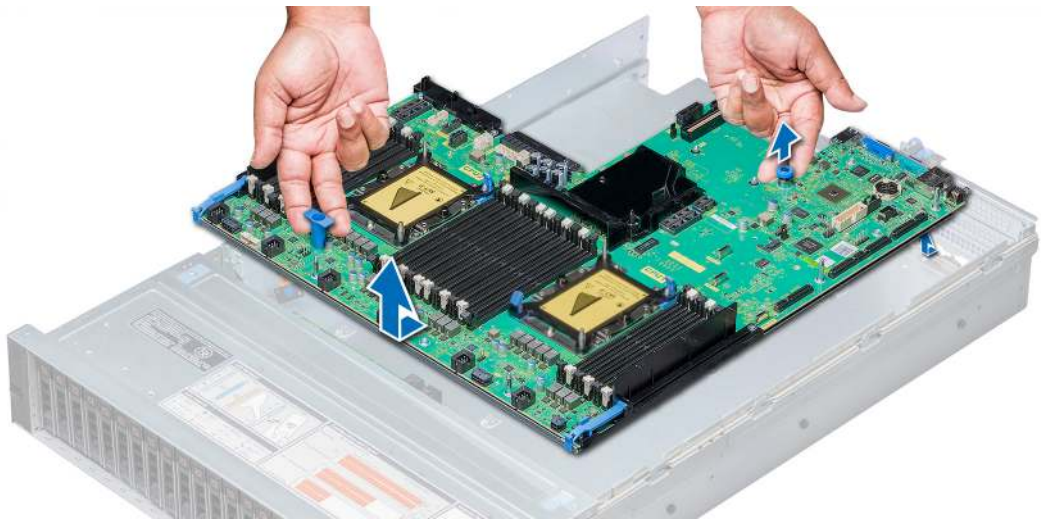
Figure 131. Removing system board
