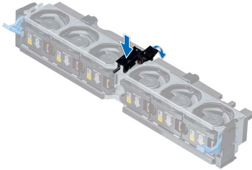
Figure 39. Installing an intrusion switch
