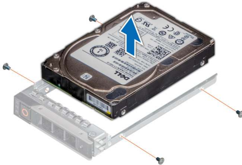
Figure 54. Removing the drive from the drive carrier
