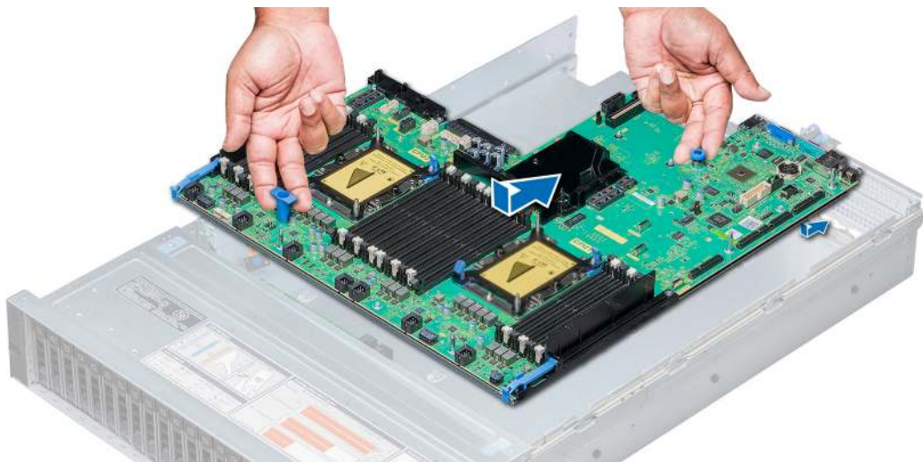
Figure 132. Installing system board
