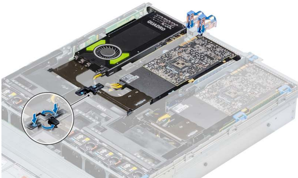
Figure 96. Securing GPU 2 and 3
