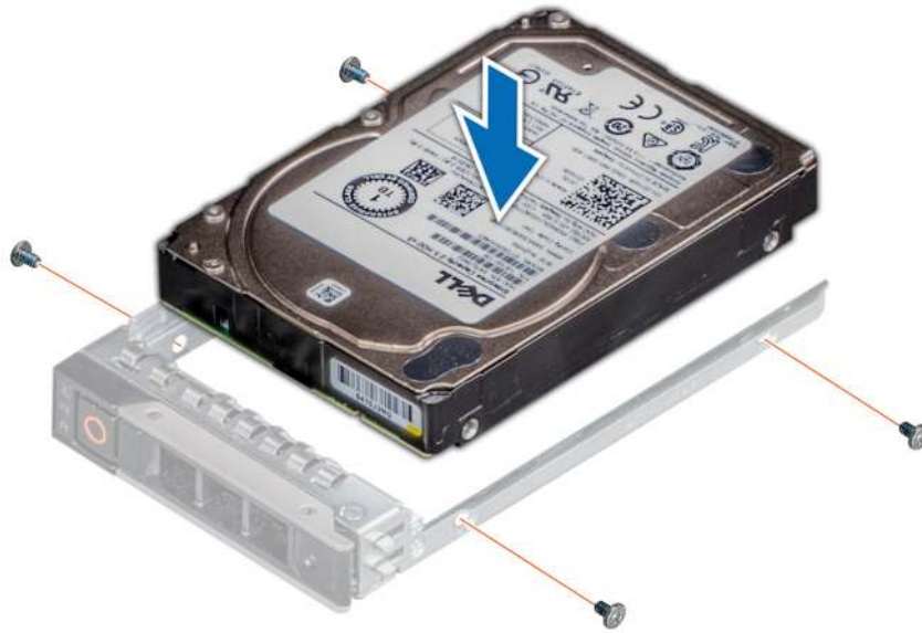
Figure 55. Installing a drive into the drive carrier
