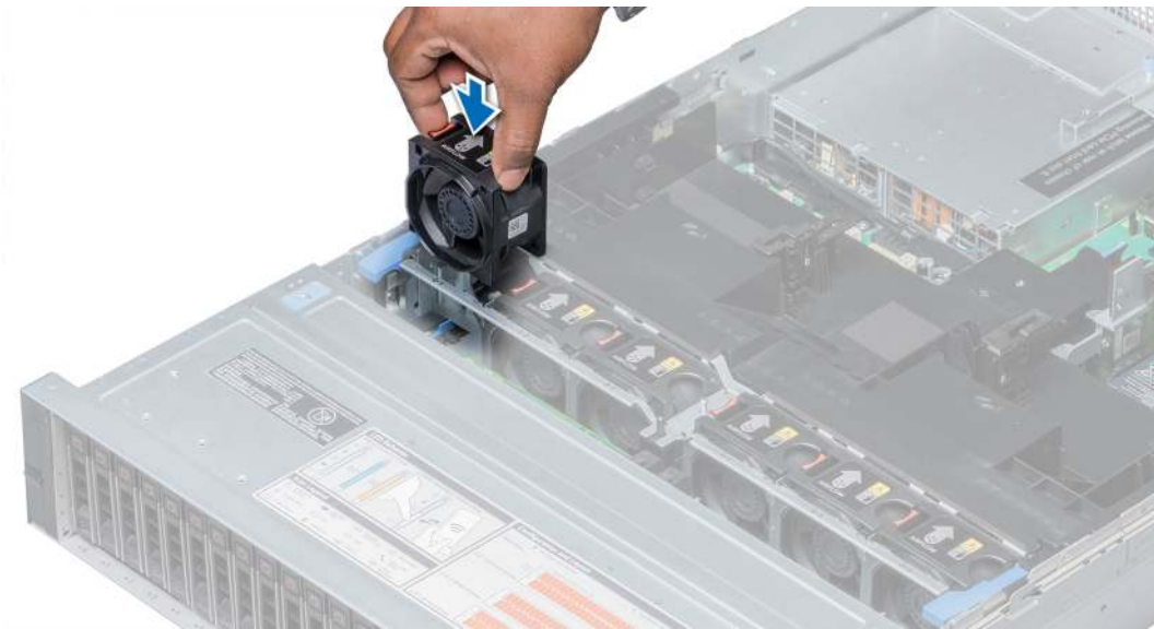
Figure 37. Installing cooling fan
