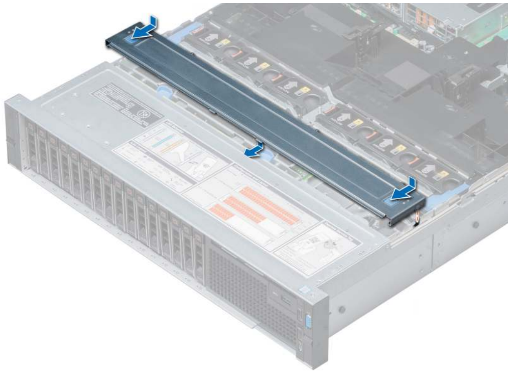
Figure 29. Installing the backplane cover
