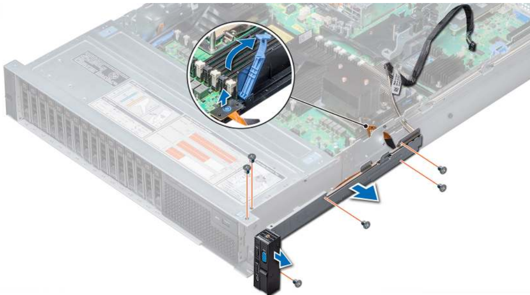
Figure 136. Removing right control panel
