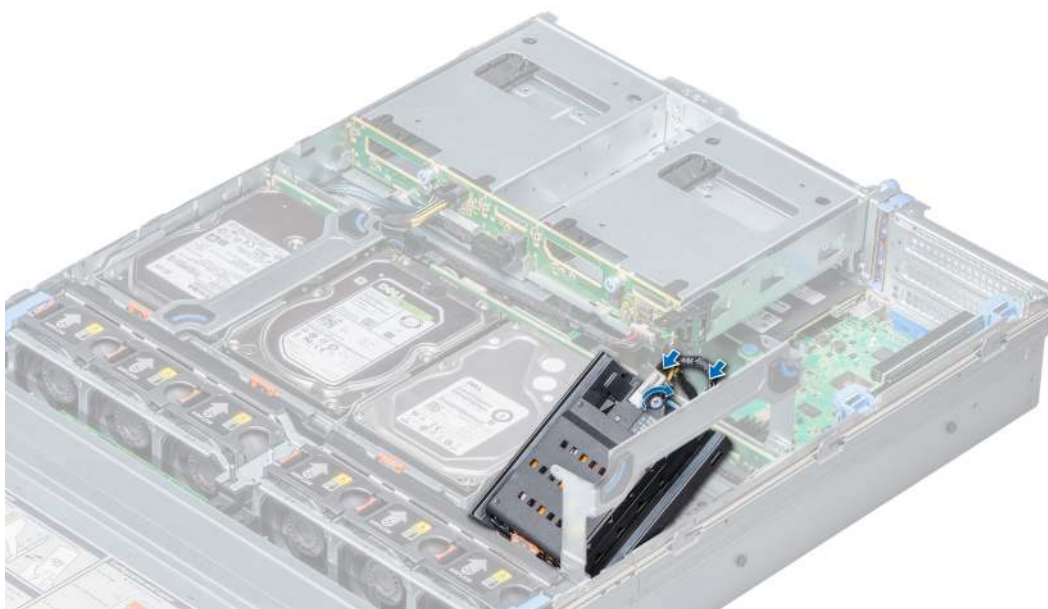
Figure 43. Installing NVDIMM-N battery into mid drive tray
