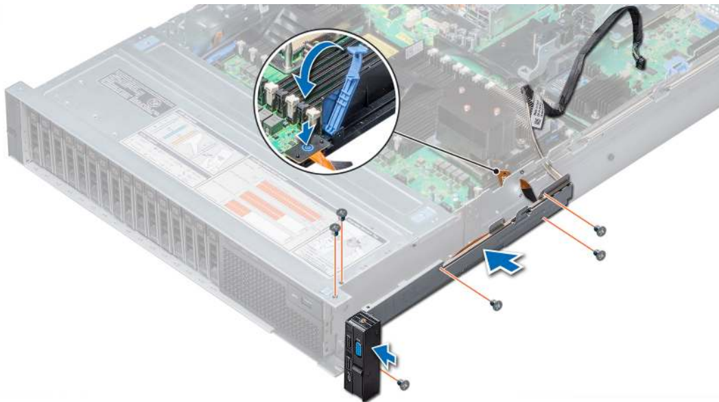
Figure 137. Installing right control panel
