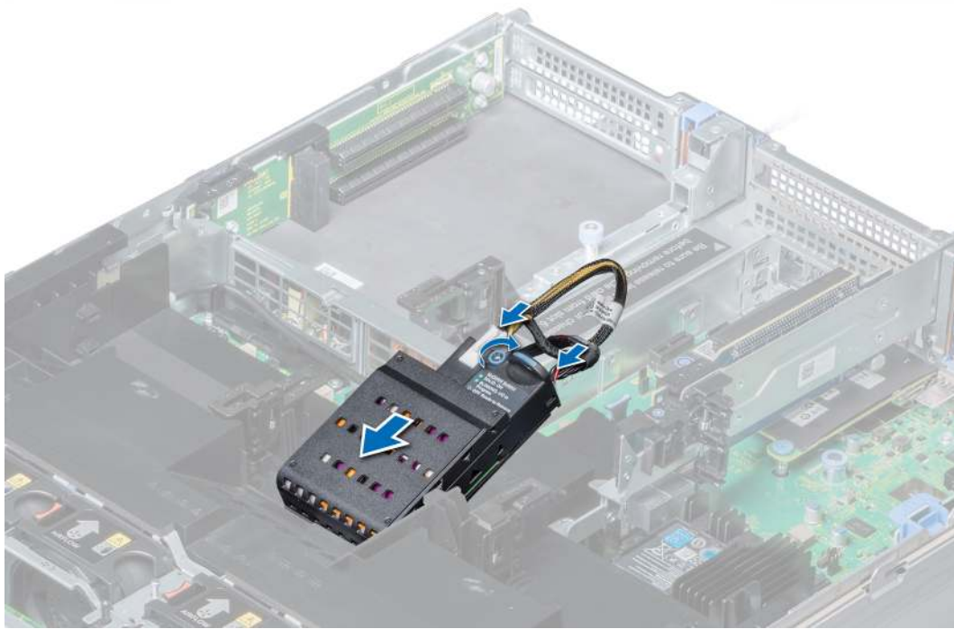
Figure 41. Installing NVDIMM-N battery into air shroud
