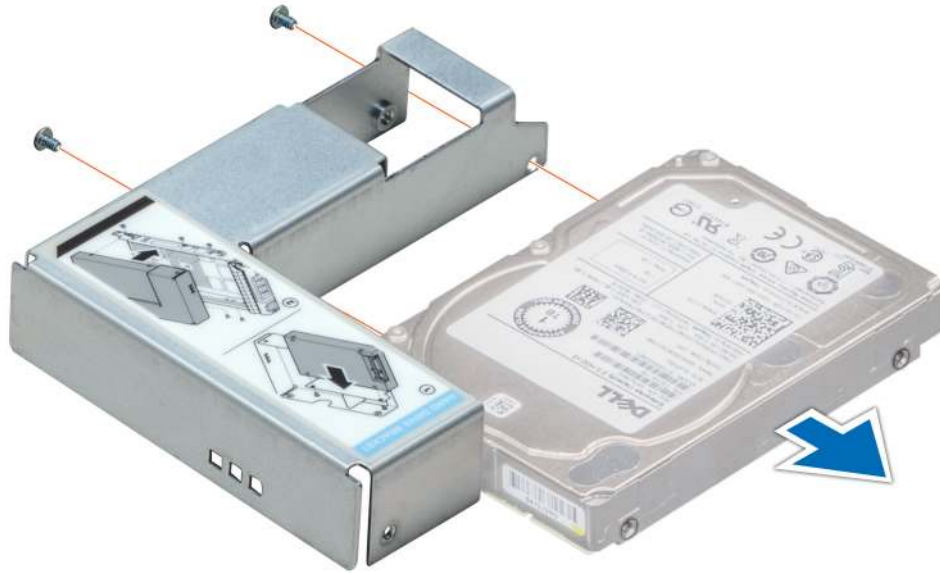
Figure 50. Removing a 2.5 inch drive from the 3.5 inch drive adapter
