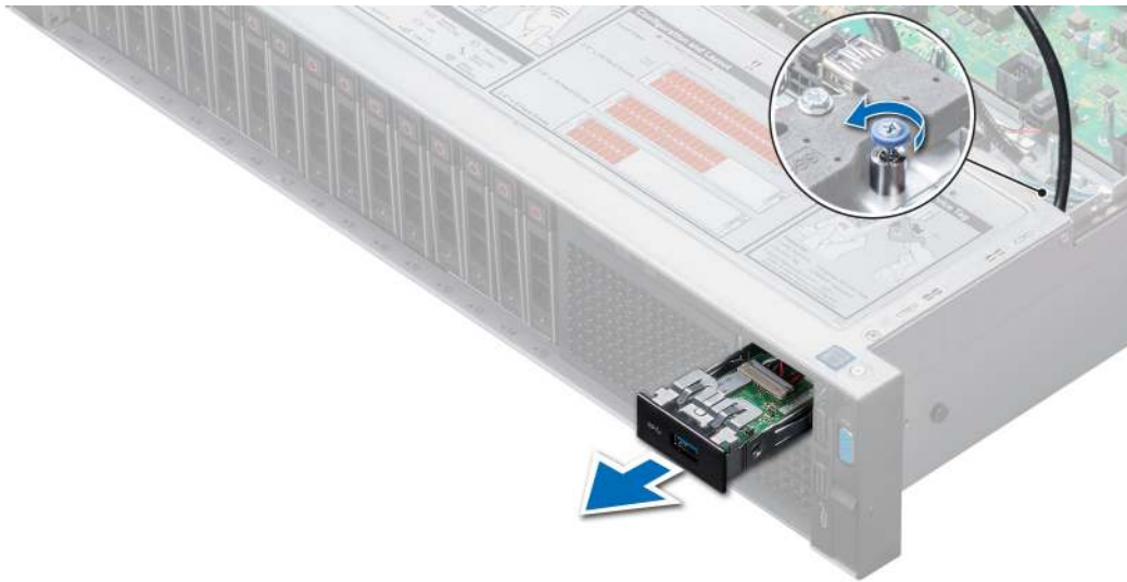
Figure 123. Removing USB 3.0 module
