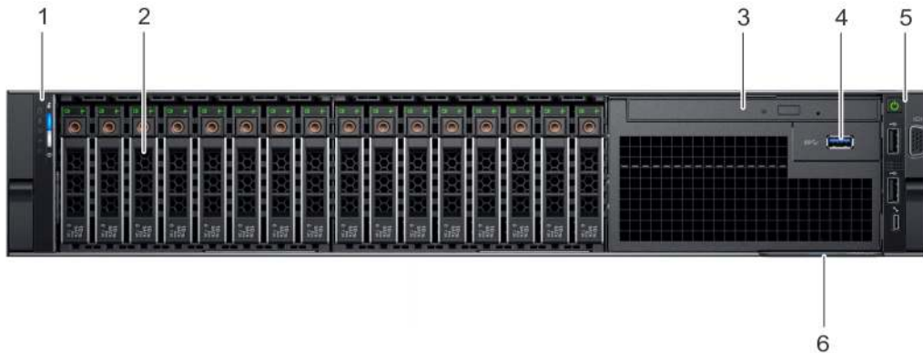
Figure 2. Front view of 16 x 2.5 inch drive system
