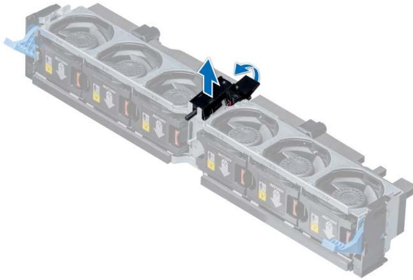
Figure 38. Removing an intrusion switch
