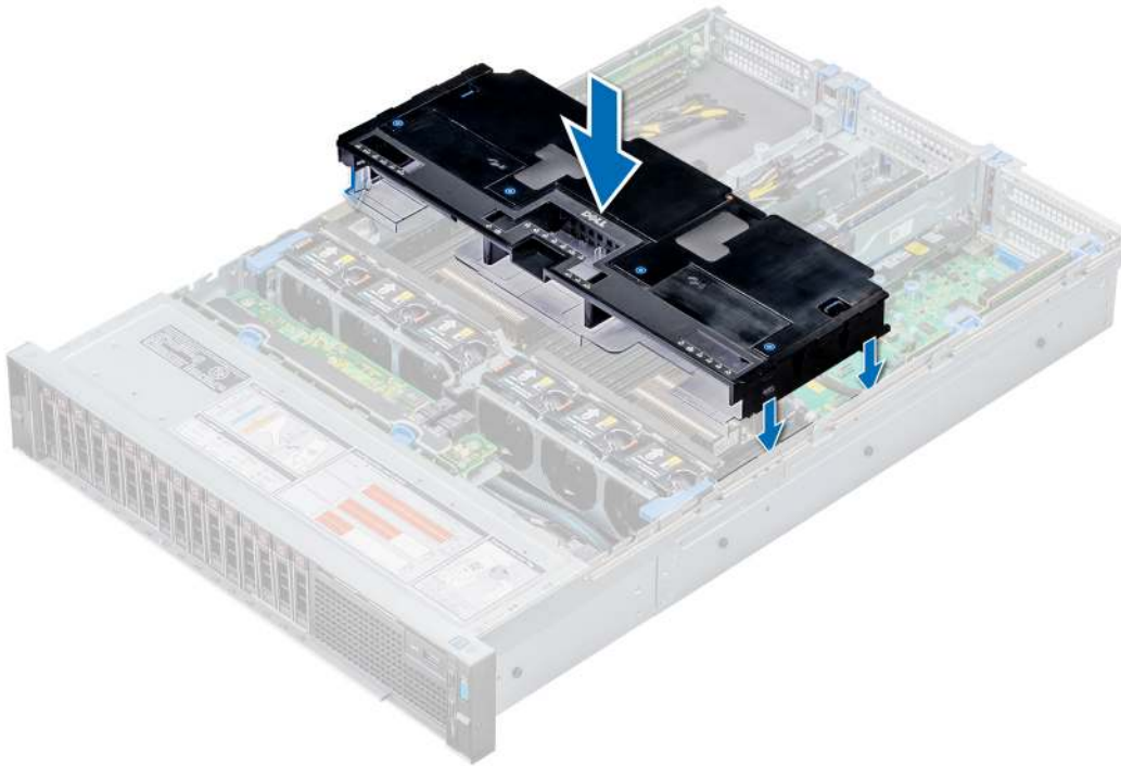
Figure 90. Installing GPU air shroud
