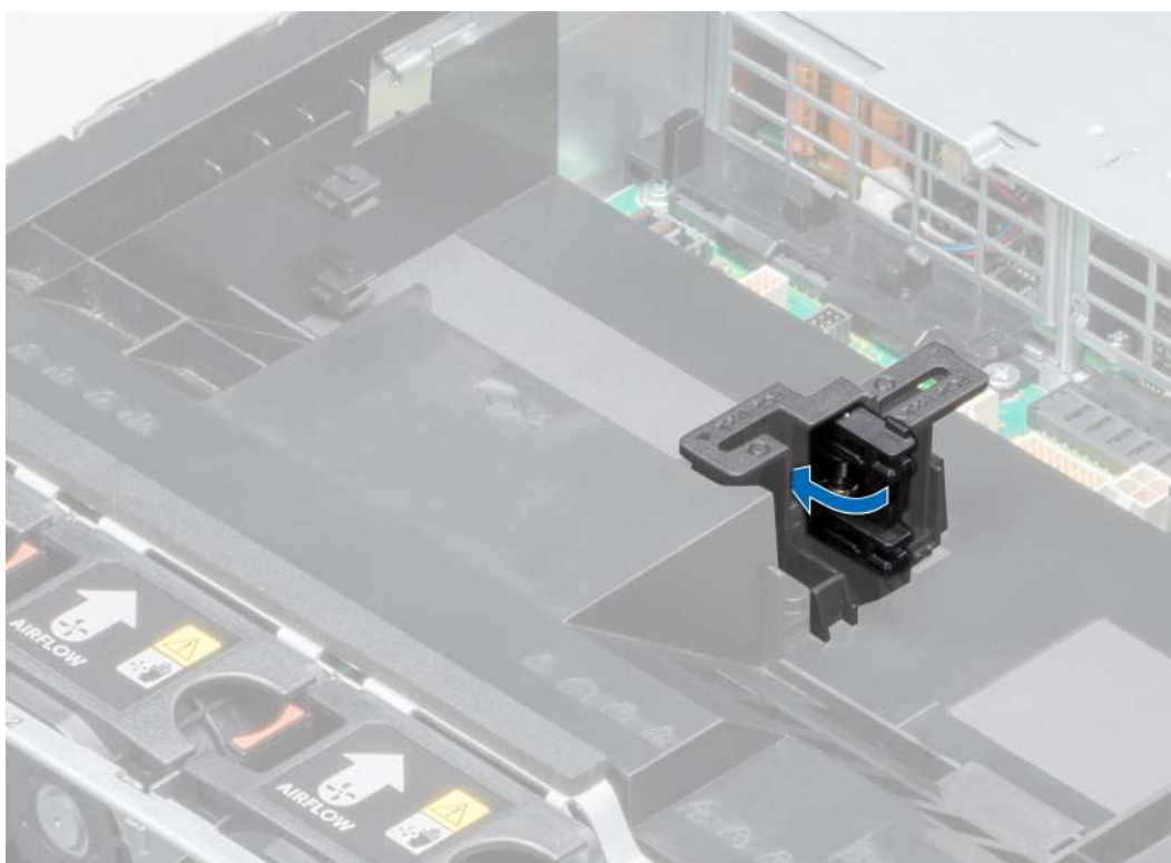
Figure 66. Closing the PCIe card holder latch
