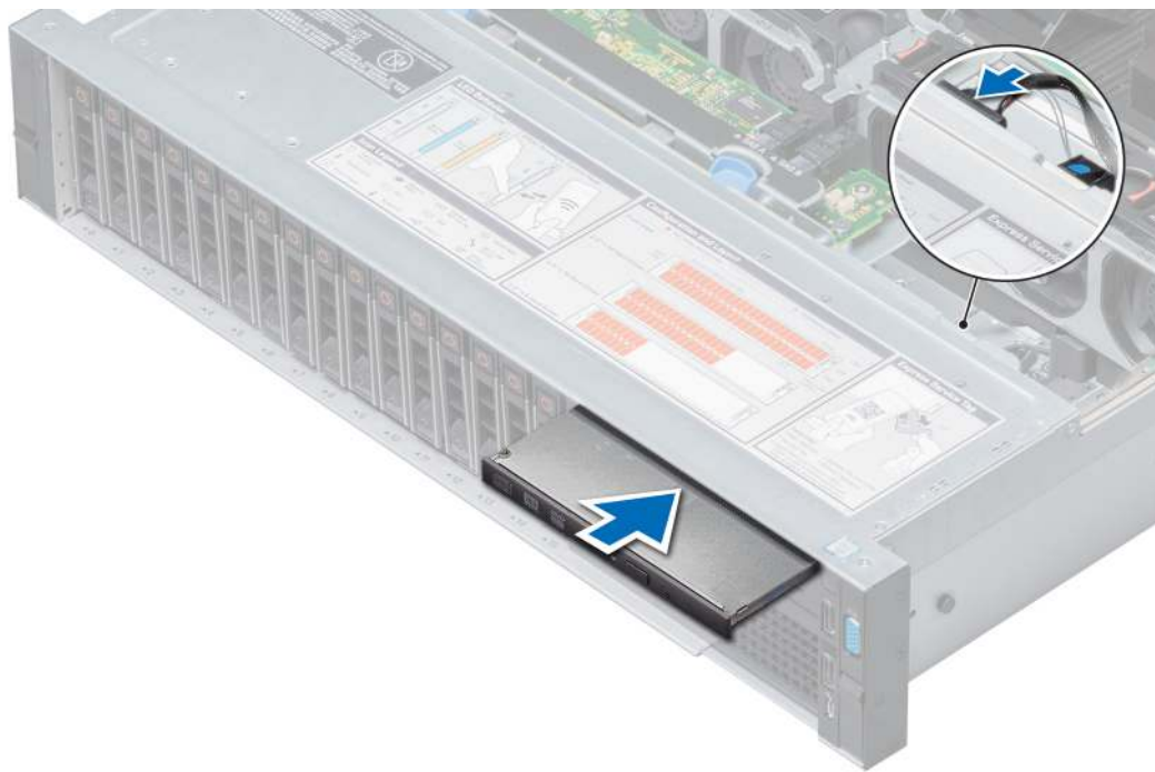
Figure 126. Installing the optional optical drive
