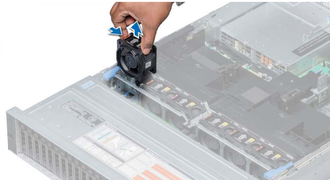
Figure 36. Removing cooling fan
