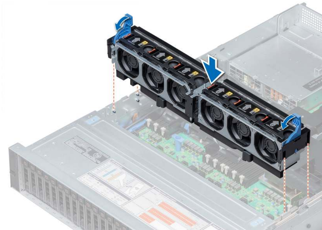
Figure 35. Installing the cooling fan assembly
