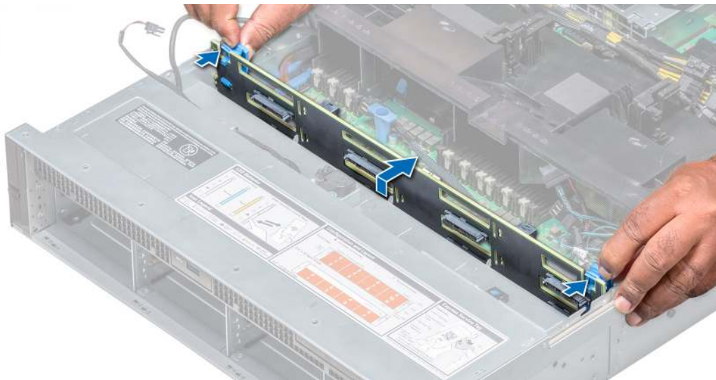
Figure 112. Removing the backplane
